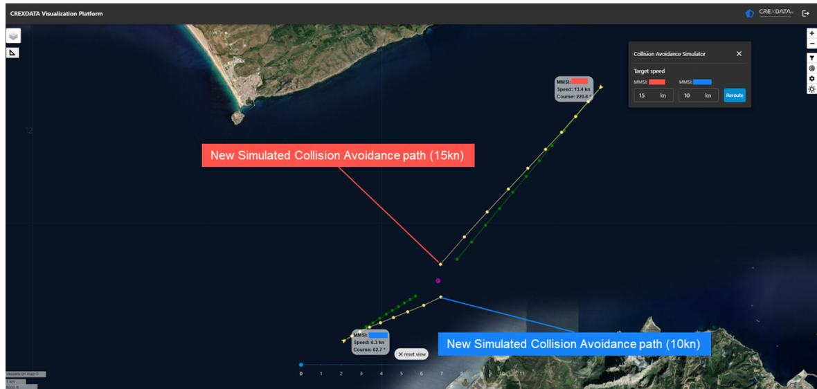
Figure 38: Output of the speed-based simulation function. In this example the operator specifies target speeds of 15 kn (red) and 10 kn (blue) for the two vessels as the forecasted collision positions lies too far ahead. The simulator computes new collision-avoidance paths (yellow-coloured paths) that divert the vessels around the forecasted collision point.
